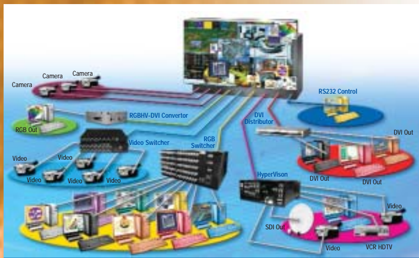
Example2: HyperCube 3 x 2 with several channels connected to direct cameras, HyperVisions, 2 external switchers (1 video and 1 RGB) and Converters and DVI distributors.
